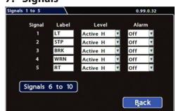
**Label**: For signals 1-5, select from: LT left turn, STP stop, BRK brake, WRN warning light, and RT right turn. Labels can be edited.
